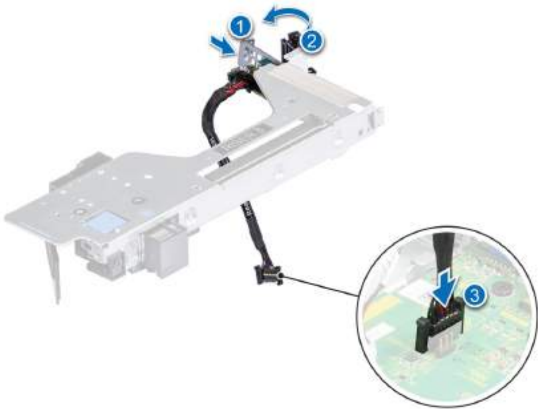
Figure 150. Installing the serial COM port
