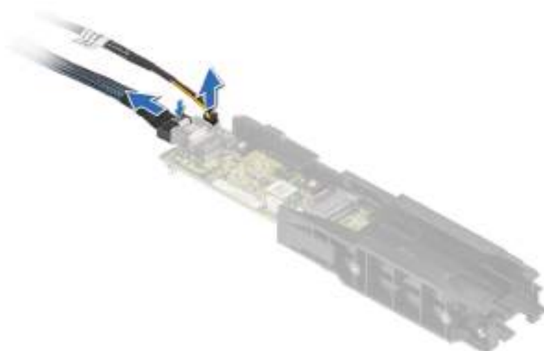
Figure 158. Removing the BOSS-N1 power and signal cable from the BOSS-N1 module
