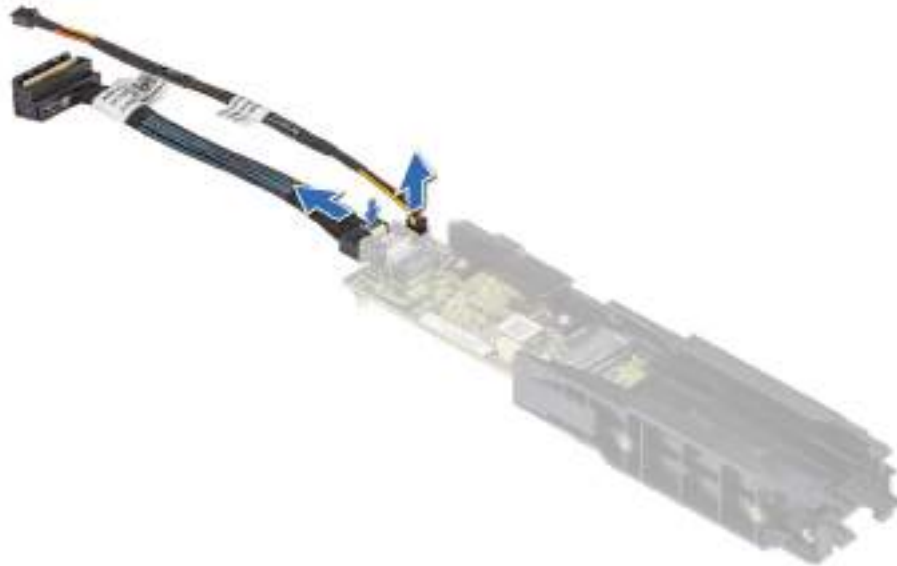
Figure 125. Removing the BOSS power cable and signal cable from the controller card module
