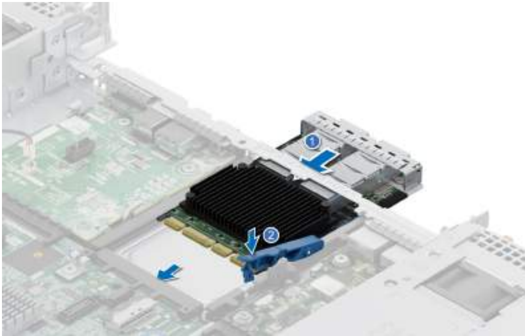
Figure 174. Installing the OCP card
