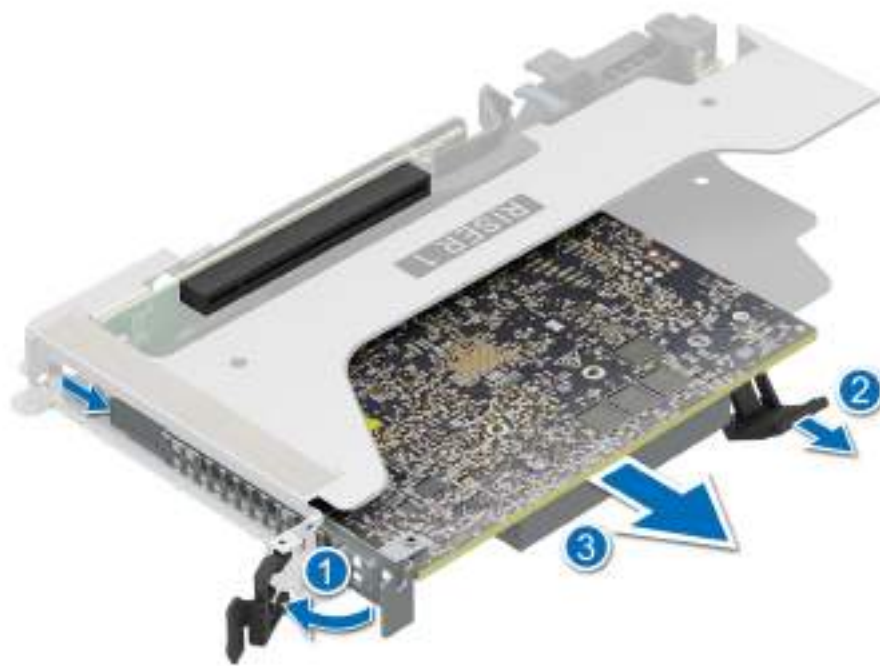
Figure 142. Removing expansion card from the expansion card riser
