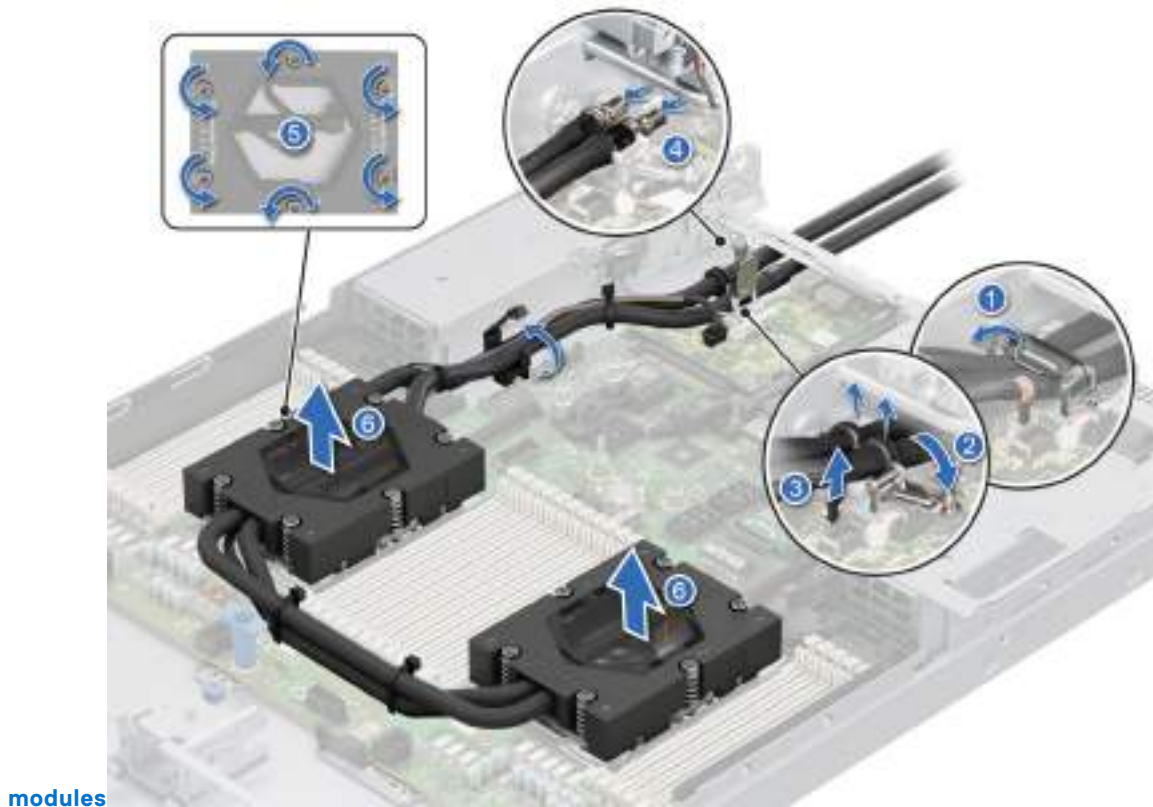
Figure 113. Removing the liquid cooling heat sink
