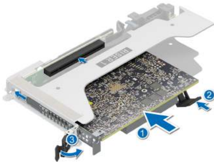
Figure 146. Installing an expansion card into the expansion card riser
