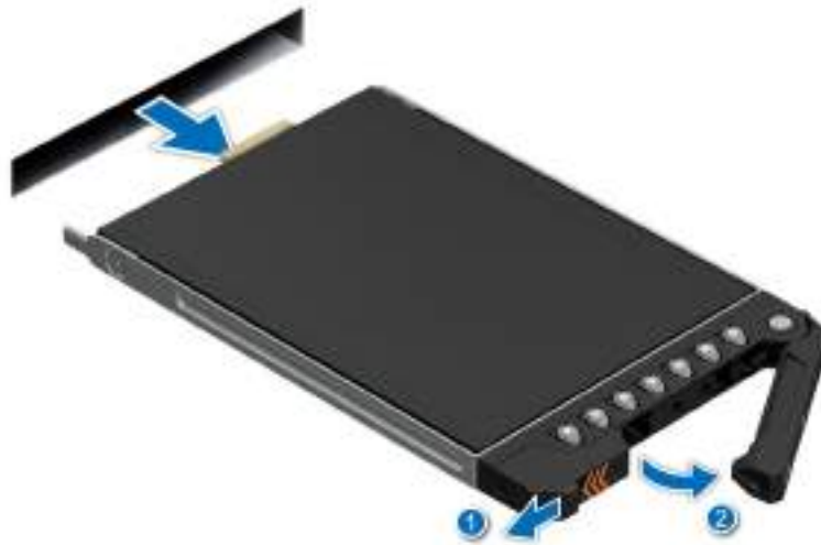
Figure 52. Removing a E3.S drive carrier
